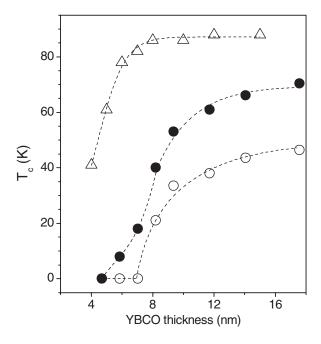
FIG. 2. Superconducting transition temperature  $(T_c)$  as a function of YBCO thickness for samples that are fully oxygenated in the dark (open triangles), deoxygenated in the dark (open circles), and deoxygenated during illumination (solid circles). Lines are guides to the eye.  $T_c$  is depressed for oxygen deficient bilayers. Notice the  $T_c$  enhancement for bilayers with YBCO thickness larger than 4 u.c.
