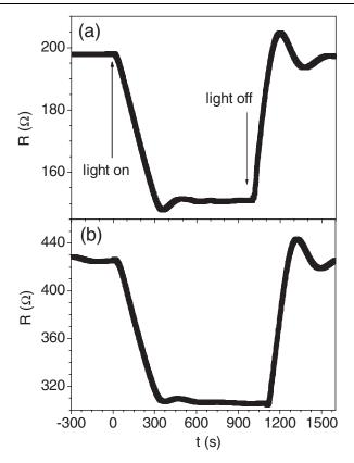
FIG. 3. Time dependence of the resistance when the light is switched on (t = 0 s) and off for (a) a 12 u.c.YBCO<sub>6.7</sub>/40 u.c.LCMO bilayer, and (b) a 60 u.c. LCMO film, both at T = 100 K. The relaxation times for the bilayer and the single LCMO film are similar and show that the effect is *transient* even at low (100 K) temperatures.
