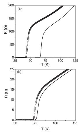
FIG. 1. (a) Resistance curves vs temperature for a bilayer with 12 u.c. YBCO<sub>6.7</sub>/40 u.c. LCMO, in the dark (open symbols) with  $T_c = 43$  K, and under illumination (solid line). The change in the critical temperature is  $\Delta T_c = 23$  K. (b) Resistance curves for a single YBCO<sub>6.7</sub> thin film in the dark (open symbols) and during illumination (line). The enhancement of  $T_c$  under illumination is 3.6 K.
