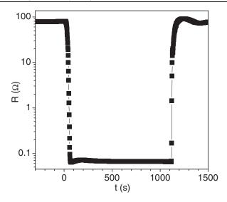
FIG. 4. Time dependence of the resistance for a 12 u.c. YBCO<sub>6.7</sub>/40 u.c. LCMO bilayer at T = 50 K signaling the transition from the metallic to the superconducting state under illumination. The effect is *transient*, since even at low temperatures the initial value of the resistance is recovered on a short time scale when the light is turned off.
